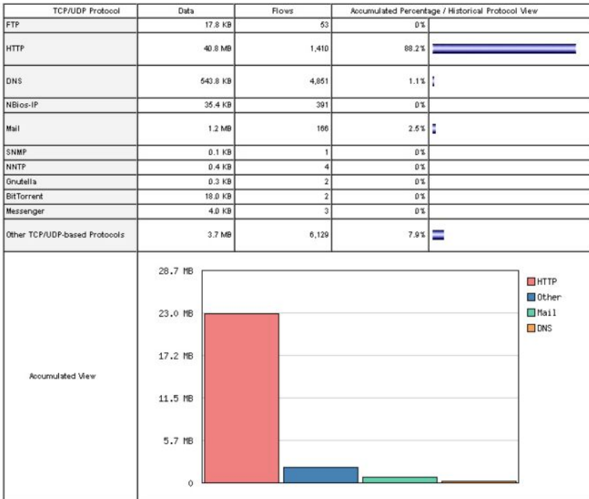
Figure 3.20: ntop displays a wealth of information about how your network is utilised by various clients and servers.
